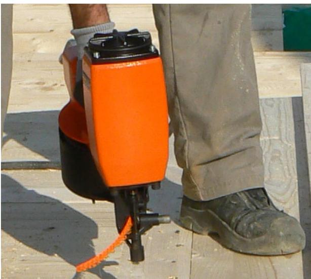
**Figure 10:** Nailing in horizontal position
