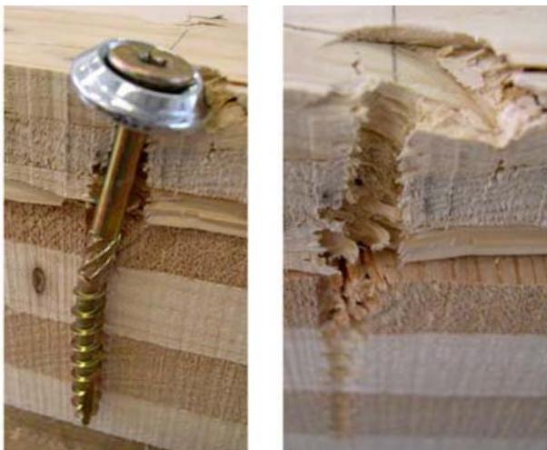
**Figure 12:** C-type sample after the test
