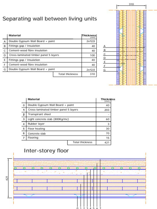
**Figure 4:** Detail of the separating wall between living units and of the inter-storey floor.
