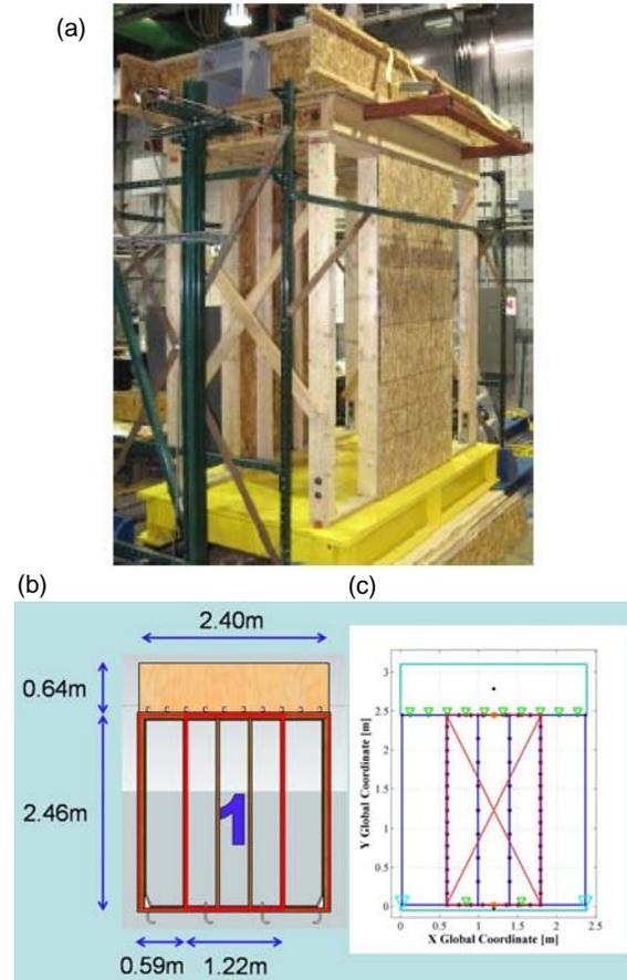
**Figure 8:** (a) Photo of the Test Specimen (after [15]) (b) Geometric and Panel Configuration; and (c) Numerical Model of the RPI Wall.
