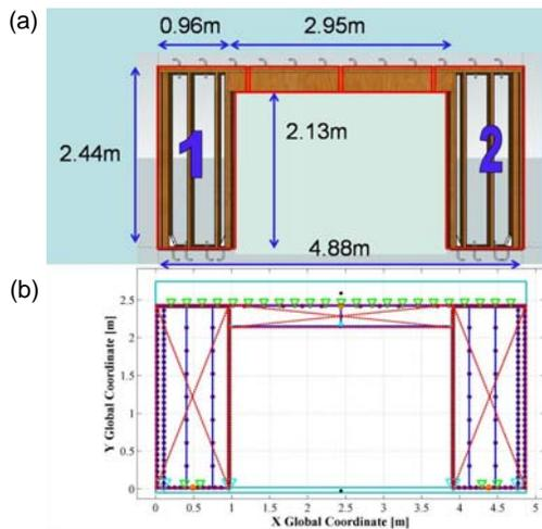
**Figure 3:** (a) Geometric and Panel Configuration; and (b) Numerical Model of the GD Wall.
