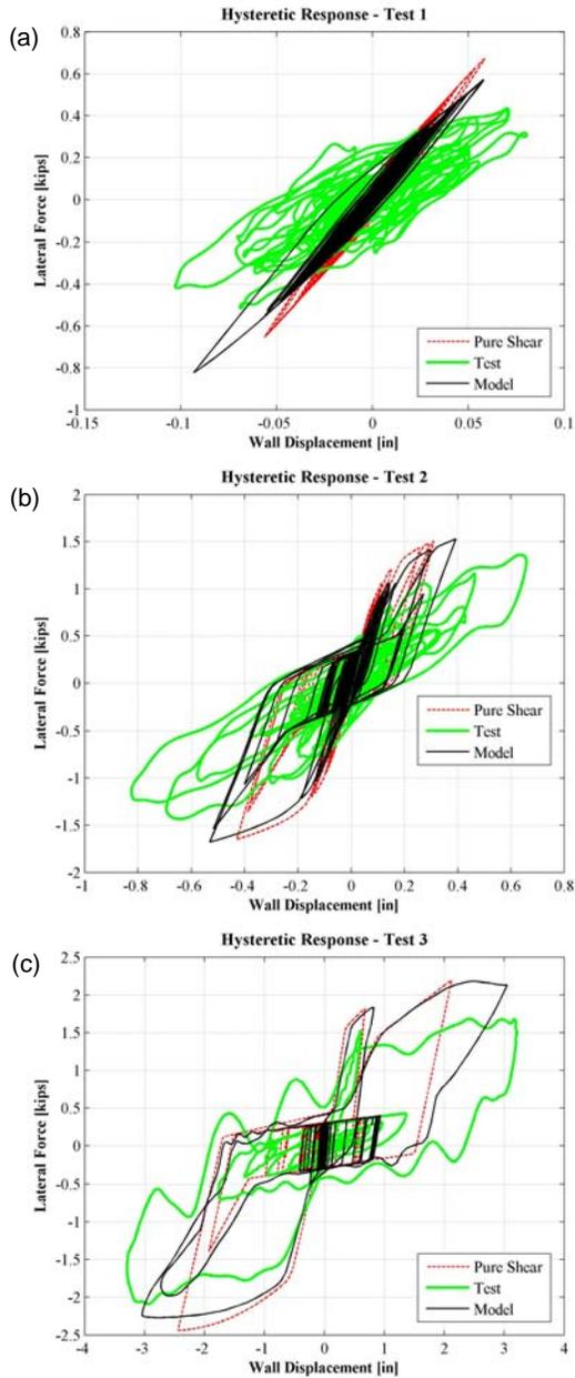
**Figure 10:** Hysteretic Response of the RPI Wall for (a) Test 1; (b) Test 2; and (c) Test 3.
