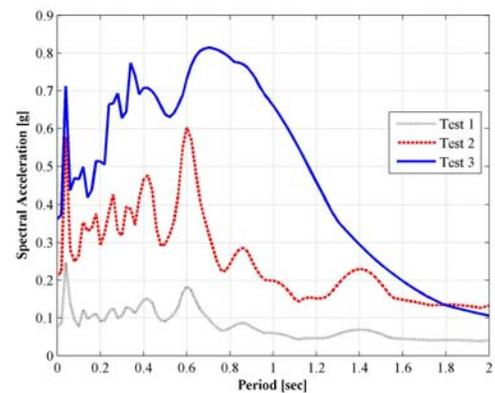
**Figure 9:** Acceleration Response Spectra of the Achieved Input Ground Motions
