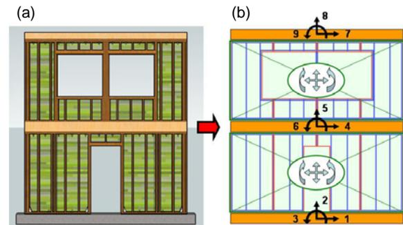
**Figure 1:** (a) Typical Exterior Wall of a Two-Story Light-Frame Wood Building; and (b) Illustration of Master DOF of a Building Model and Shear Wall Sub-Structures for the Simulation of Each Story.
