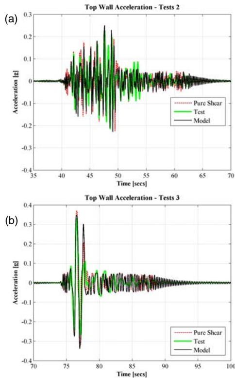
**Figure 13:** Top of Wall Acceleration of the RPI Wall for (a) Test 1; and (b) Test 2.
