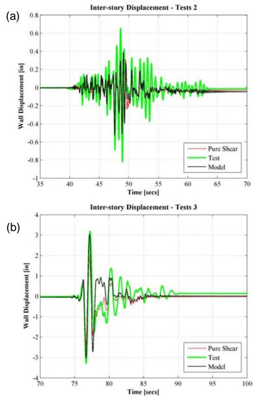
**Figure 11:** Inter-story Displacement of the RPI Wall for (a) Test 1; and (b) Test 2.
