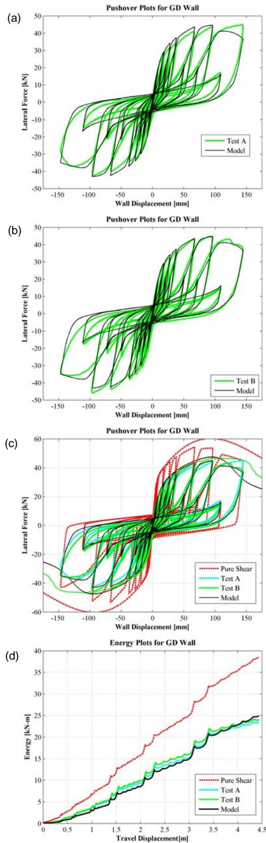
**Figure 4:** (a, b, c) Comparison of Cyclic Response; and (d) Dissipated Energy for GD Wall.
