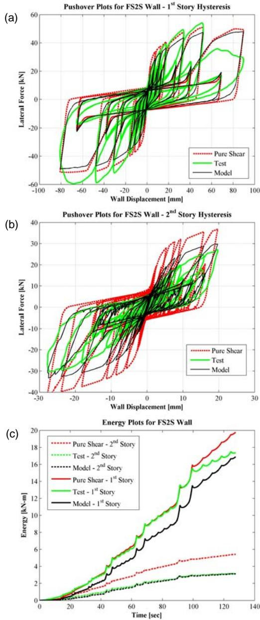
**Figure 7:** Comparison of Cyclic Response for (a) the First Story; and (b) the Second Story of FS2S Wall.
