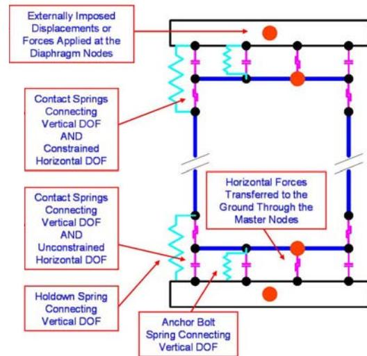
**Figure 2:** Detailed Numerical Model of the Framing Domain.
