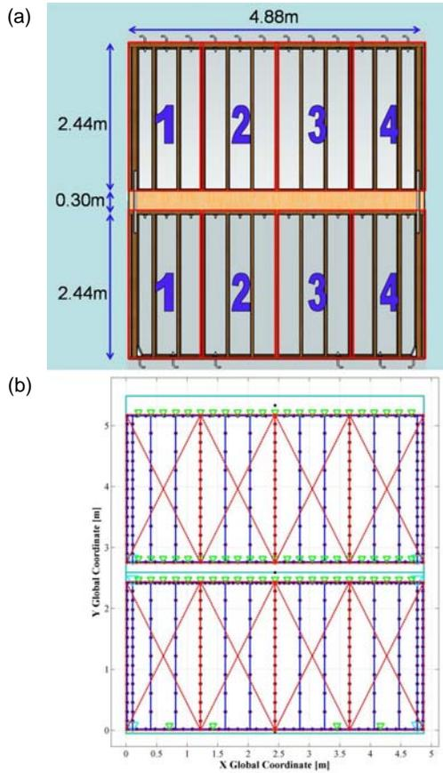
**Figure 5:** (a) Geometric and Panel Configuration; and (b) Numerical Model of the FS2S Wall.
