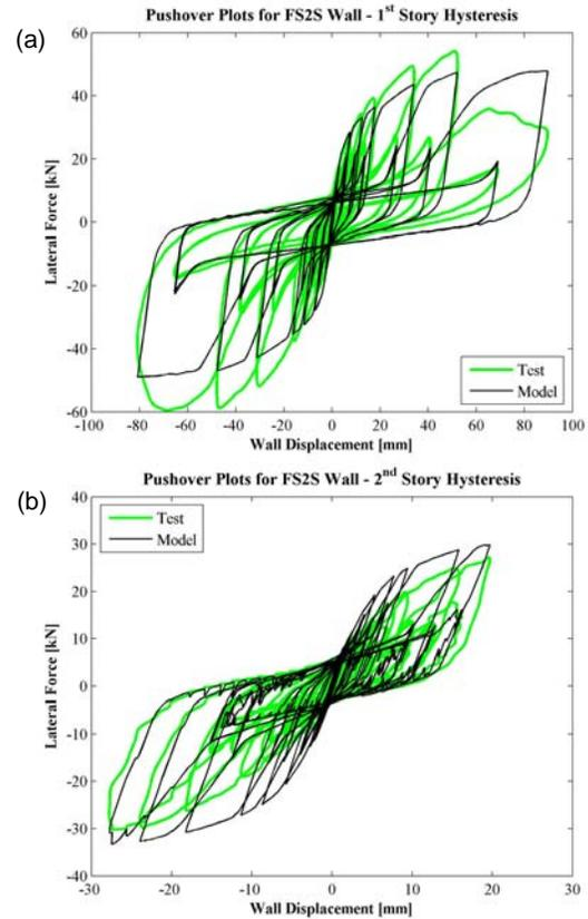
**Figure 6:** Comparison of Cyclic Response for (a) the First Story; and (b) the Second Story of FS2S Wall.
